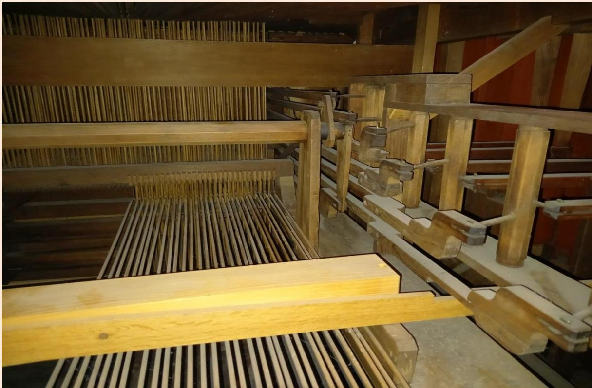
The key- and stop action is traditional made with wooden rollers and frames, trackers and metal arms and metal wiring. The nuts are from leather, pivot points are partly provided with cloth.
